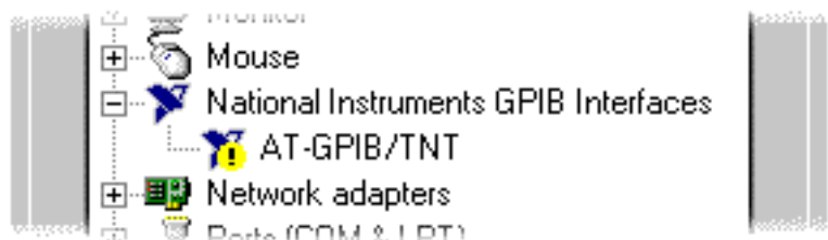
Figure C-1. GPIB Interface That Is Not Working Properly
