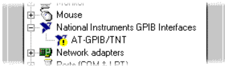
Figure 2-16. GPIB Interface That Is Not Working Properly
